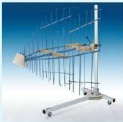
ISO 11452-2 ALSE Antennas Electric field strength
