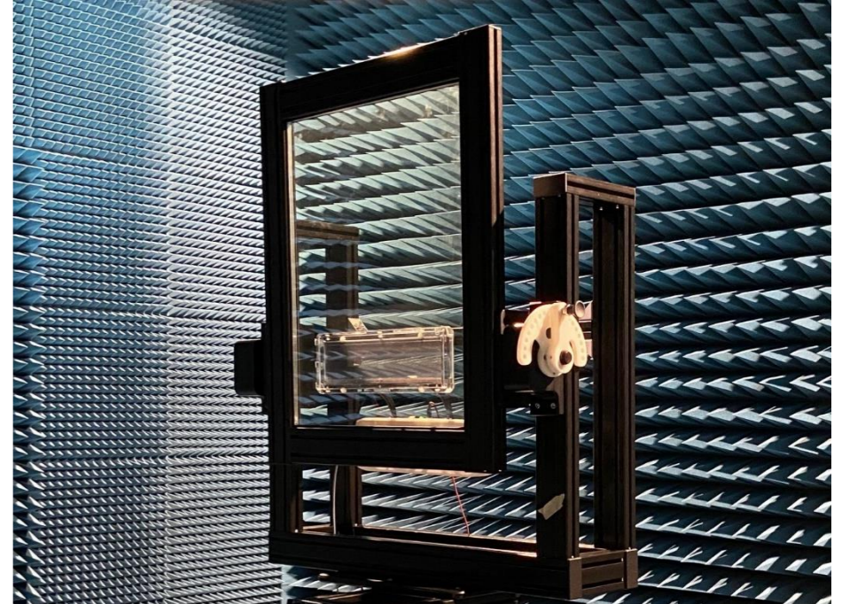
Transparent Phased Array Antenna Installed on a double glaze low-E glass setup
