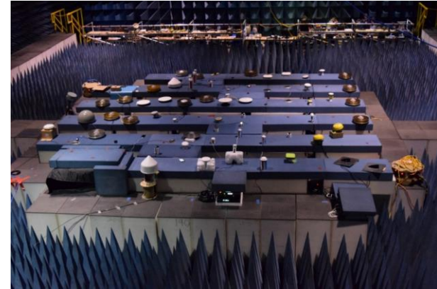
GPS/GNSS receiver test at White Sands Missile Range Anechoic Chamber (courtesy US Army)
