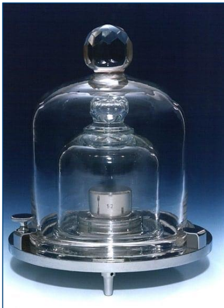
Copy of the original kilogram („Le grand K”, Paris 1889) at the PTB (German National Metrology Institute): 90% platinum, 10% iridium.
