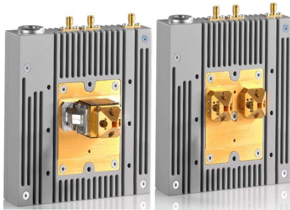
AREG8-81S/81D mm-Wave horn antenna frontends (DFF chamber)
