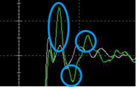
Clips have an influence on accuracy especially at full bandwidth (e.g. 200 MHz)
