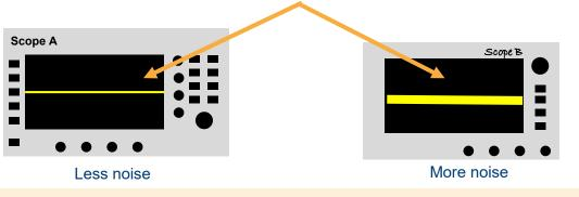
Intrinsic measurement noise with all input signals disconnected.
