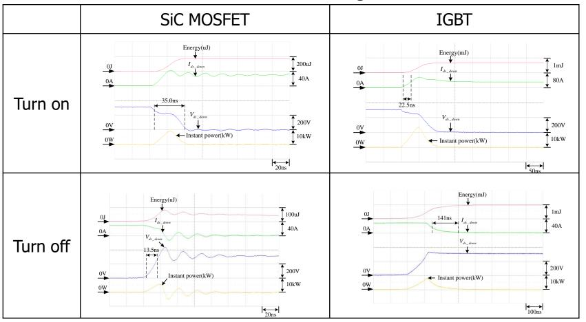
Switching loss of the SiC MOSFET and IGBT are 253.2µJ and 1597.0µJ, respectively.
