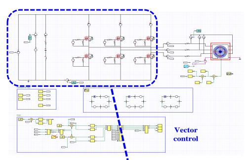
**Estimate losses of power stage** under required driving cycle and output power by Spice model using co-simulation for thermal design
