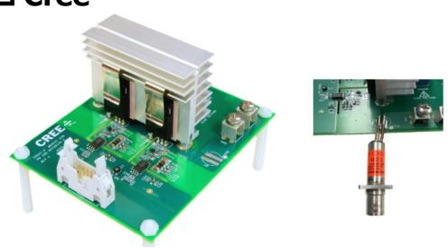
Source: Evaluation Board for Cree's SiC MOSFET in a TO-247-4 Package
