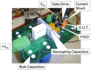
Source: High Temperature Characterization and Analysis of Silicon Carbide (SiC)
