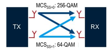
Unequal Modulation (UQAM) e.g. 2ss, [256-QAM, 64-QAM] e.g. 4ss, [1K-QAM, 1K-QAM, 256-QAM, 64-QAM]
