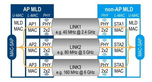
Each link enables **channel access** and **frame exchanges** between the non-AP MLD and the AP MLD based on the supported capabilities exchanged during the association.
